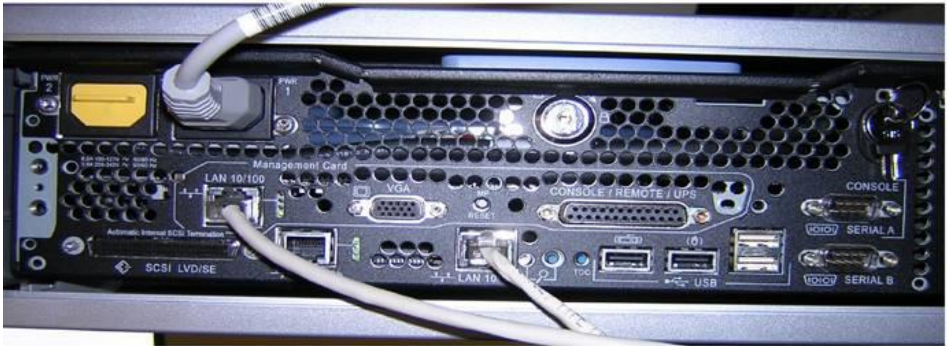
Management Processor Card MP Card 10/100 connection 1000Mb connection LAN 10/100 Management Card VGA MP RESET CONSOLE / REMOTE / UPS LAN 10 TDC USB CONSOLE SERIAL A SERIAL B Serial Console connection Three Headed Cable Connection
